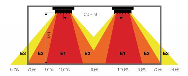
When using more than one panel within a room, it is good practice to provide an even spread and an overlap of intensity above head height.
