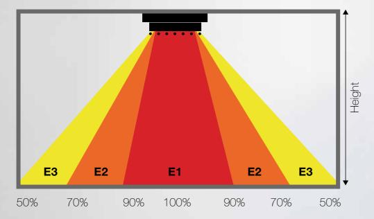
Within the radiant field itself, there are also varying levels of intensity. The diagram above shows that the area directly under the centre of the panel (E1) receives an output level of 90-100%, while the outer edge (E3) is 50% of the intensity of E1. These calculations are important when positioning panels in specific buildings.
