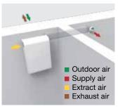
Expandable for even more flexibility. Adjoining rooms can also be integrated into the ventilation system as a result of the adjoining room connection. Large residential units can use several units to supply and extract air.
